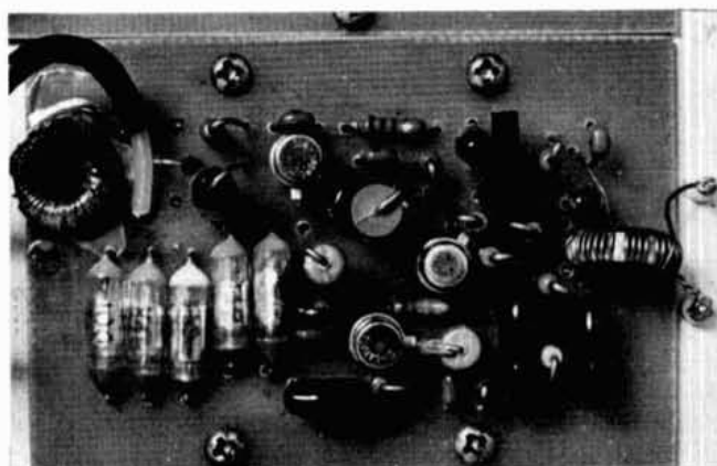
The VFO board. Note coax connection to variable capacitor.
