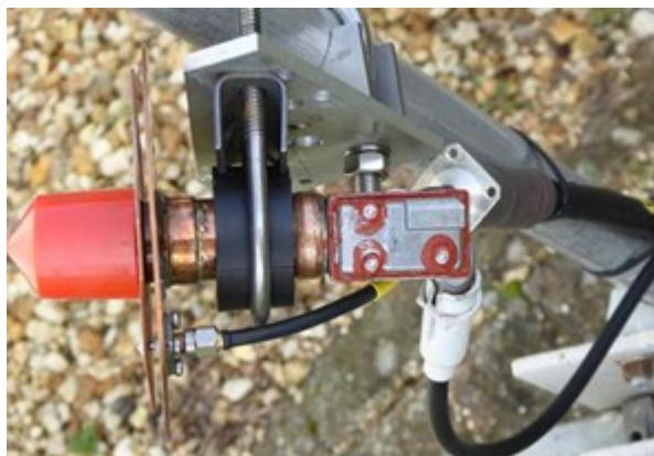
G0MJW (note olive/clamp ring behind reflector)
