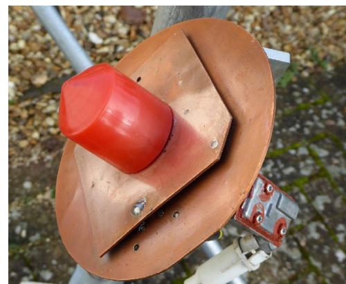
Figure 10 – Rocket LNB lens on patch
