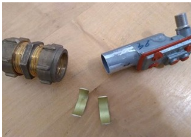
Figure 5 – Compression fitting for a decapitated LNB
